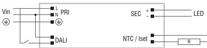
PUSH SWITCH diagram - Collegamento PUSH SWITCH
